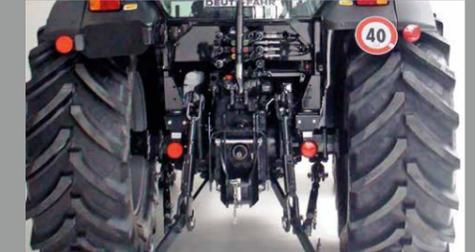
The rear power lift of the 5D Series with additional lifting cylinders lifts up to 3,600 kg and can therefore manage all common equipment in this power class.
