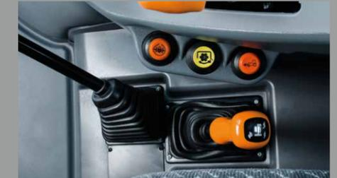
Electro-hydraulic activation of PTO, four-wheel drive and differential lock as standard (LS and GS).
