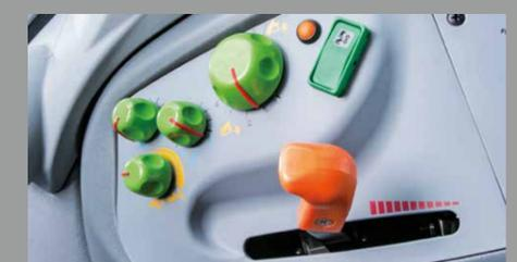
Accurate electronic hitch regulator (EHR) and electronic engine speed memory for recalling speeds during routine tasks.
