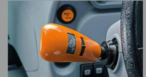
Powershuttle lever with SenseClutch and Stop&Go switch. Stop and start without using the clutch pedal.
