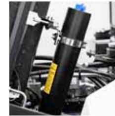
Boom suspension (Nitrogen accumulator)
