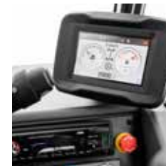
5" display with Bluetooth radio, microphone & loudspeakers
