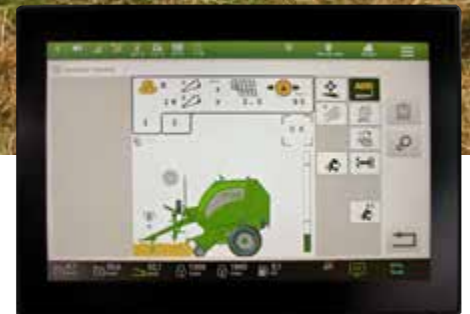
ISOBUS on a tractor terminal
